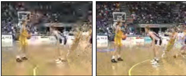
a) Non-scalable MV coding; PSNR_Y = 22.02 dB b) Scalable MV coding (PLC); PSNR_Y = 24.80 dB
